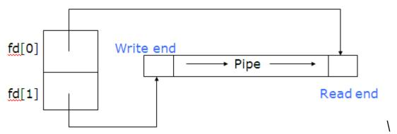
Unnamed pipes are usually used for communication between a parent process and its child, with one process writing and the other process reading.
